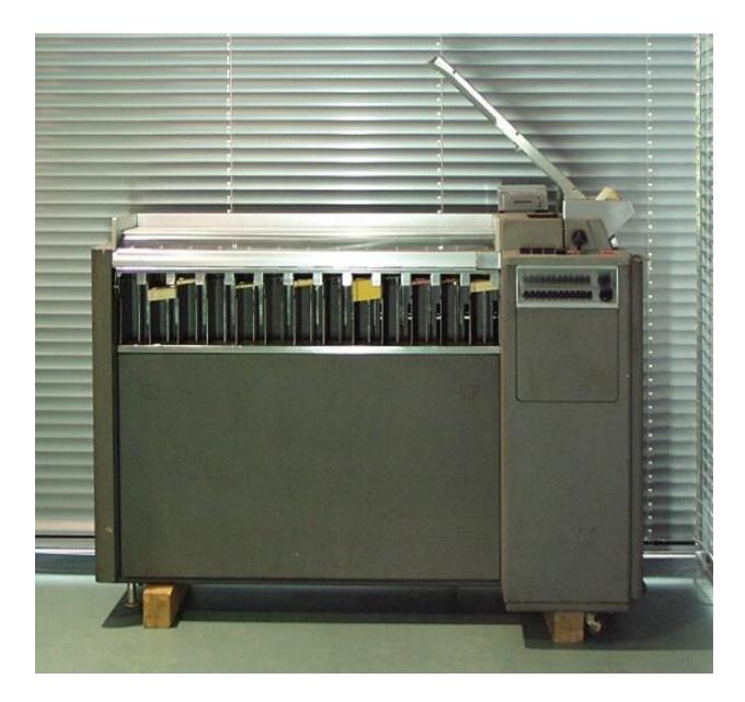
Figure 1.2: A sorting machine for punch cards.
