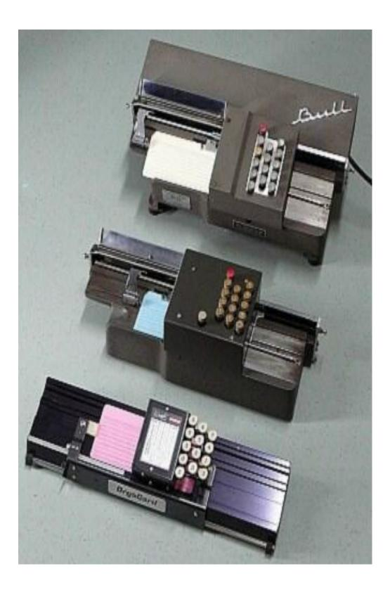
Figure 1.1 A punching device to punch holes in a punch card.
